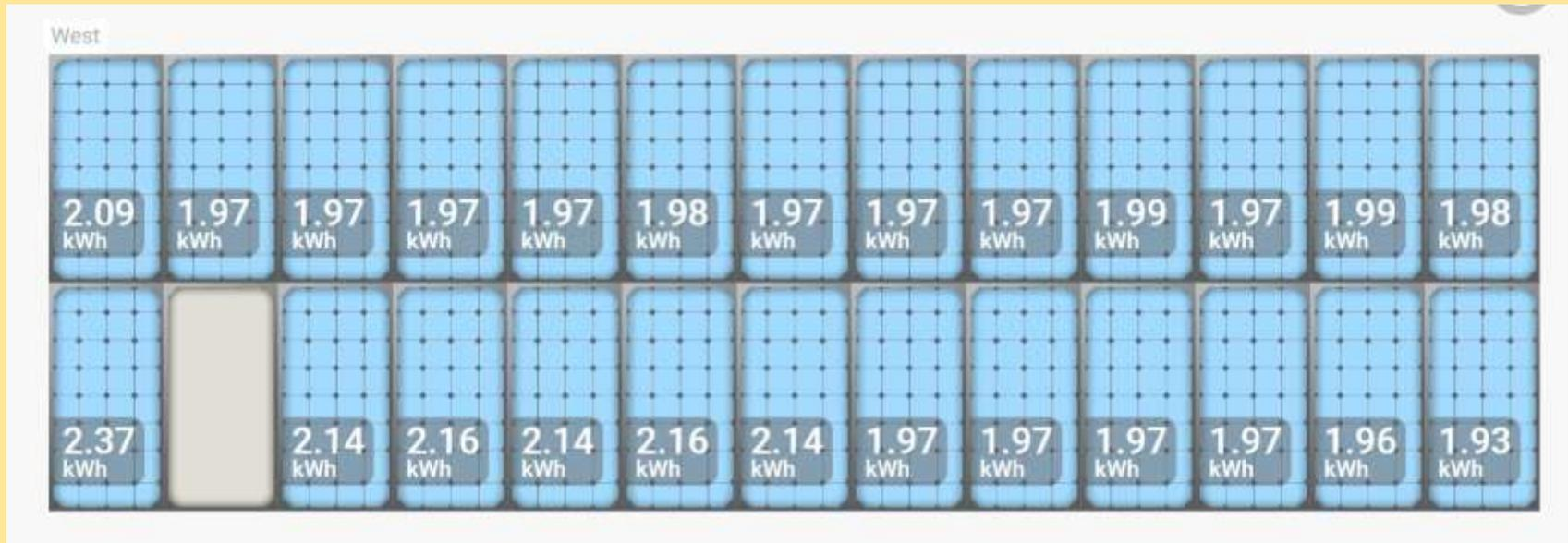
With a string inverter that one panel failure would take out an entire string. We can see that the other panels are producing and are producing consistently. All of this is via the internet.
