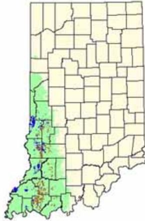
Index map of Indiana showing the coal-bearing rocks of the Pennsylvanian System in green, underground coal mines in blue, and surface coal mines in brown.
